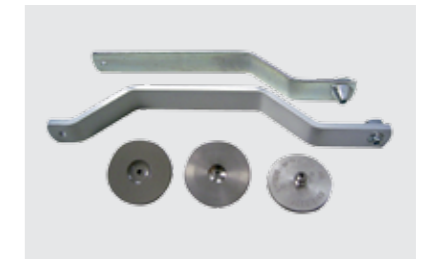
Top: Conical drilling jig, centre: drilling jig for hole = Ø 8.5 mm, bottom: rivet attachment jigs for rivet head dia. 11 and 14 mm mountable on riveting tool AccuBird (MBE)
