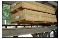
Pull the pallet carefully out of the container. The forks should be pushed carefully as far in as possible underneath the pallet.
