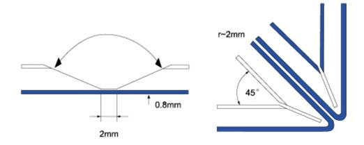
4. Rectangular groove for folding up to 150°, depends on the panel thickness.
