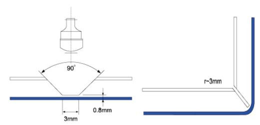
2. V-shape with flat area for folding up to  $90^{\circ}$
